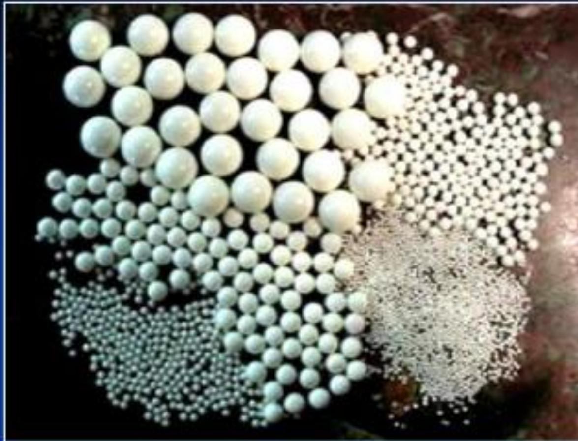
**Powders with typical particle diameters of about 50  $\mu\text{m}$  are placed together with a number of hardened steel or tungsten carbide coated balls in a sealed container which is shaken or violently agitated.**
