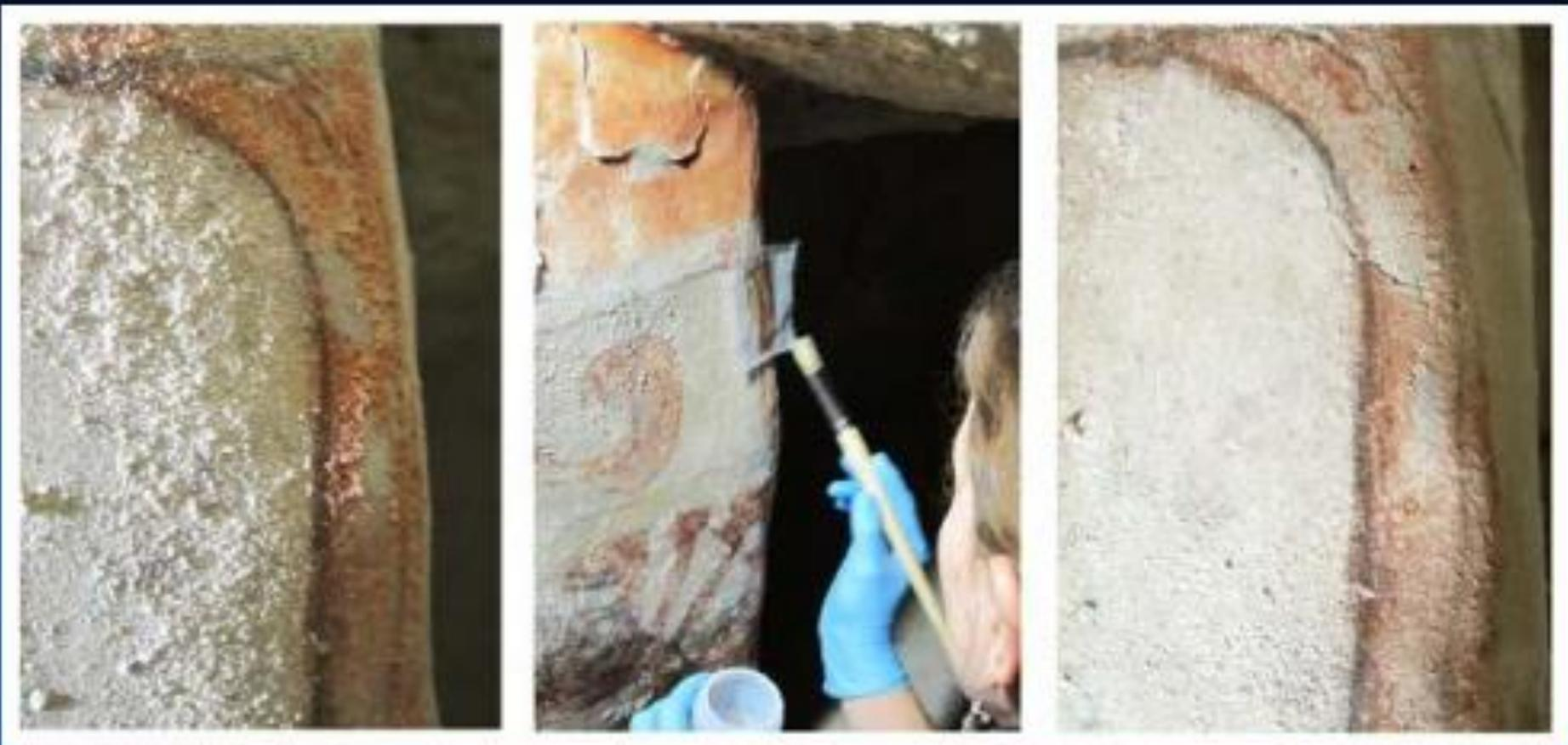
Figure 10: The restoration intervention on a pictorial surface in the archeological site of Ixcaquixtla. On the left, salt crystallization have led to the powdering of the paint layer with a consequent loss of pigments. On the center, a conservator applies  $Ba(OH)_2$  nanoparticles dispersion after the consolidation with calcium hydroxide nanoparticles and desulfation with ammonium carbonate. On the right, the same portion of the pictorial surface after the intervention.
