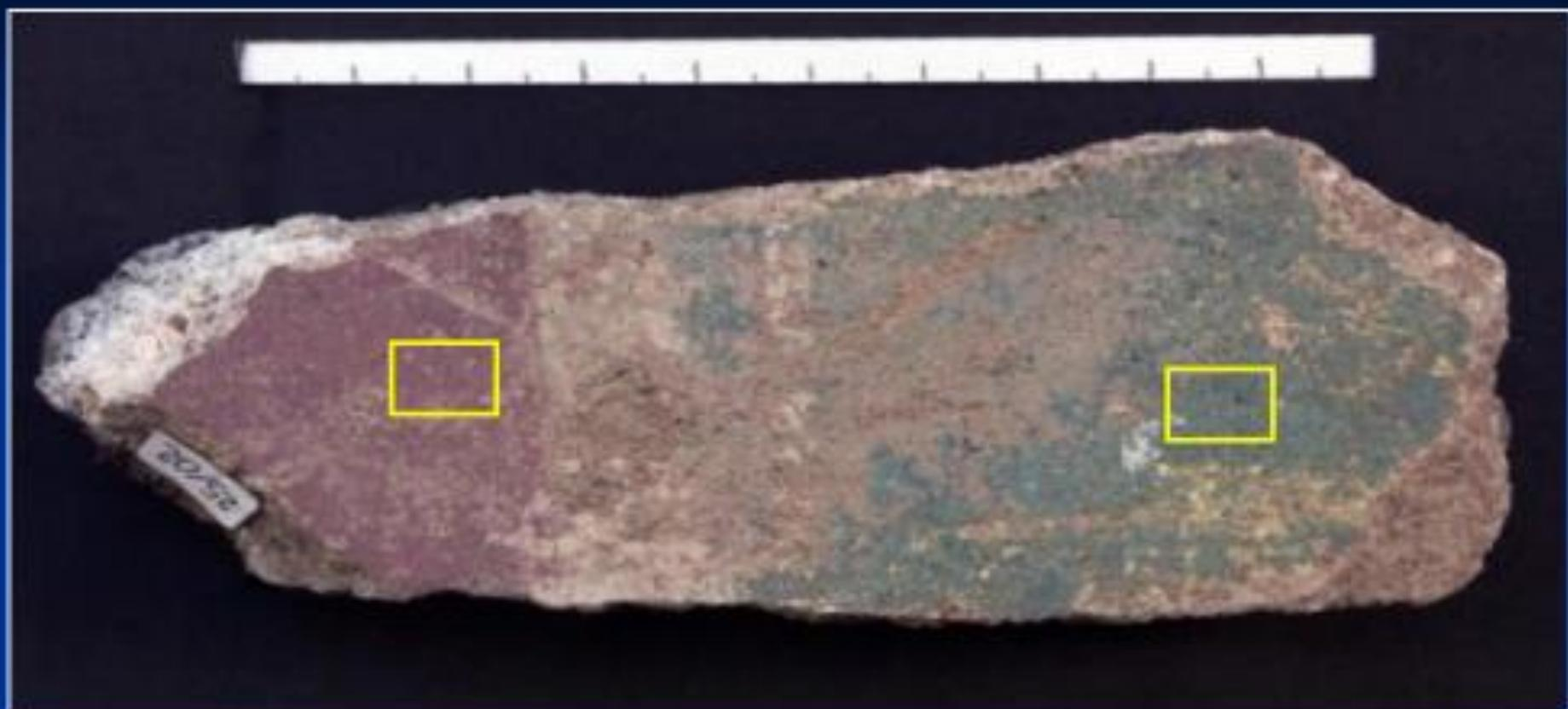
**Fig. 3.** One of the fragments of mural paintings used in the evaluation of the product. The fragments are from the House of Ariadne in Pompeii (Italy) (first century AD). Marked areas correspond to areas treated with the colloidal suspension based on barium oxide.
