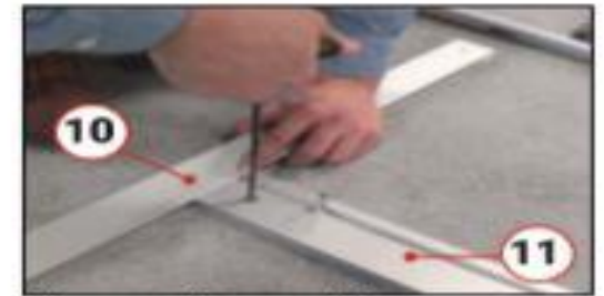
Align part #10 to part #11 and secure CAM Lock using hex key.
