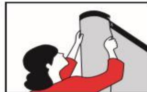
Bow endcaps and lift onto studs atop both sides of frame. For hinged panels hook one side then the other. Slide hands along length of panel to bond magnets.
