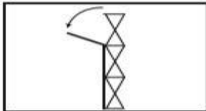
Lift top section of strut up, rotate down. Remove all lights.
