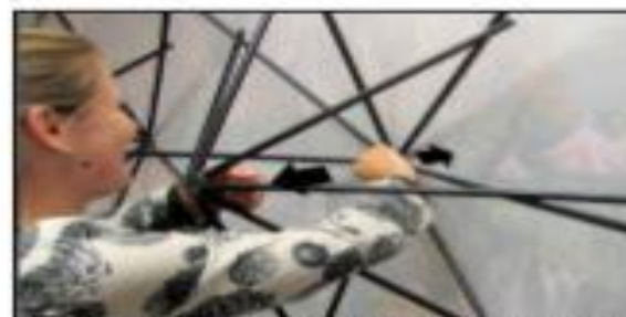
STEP 10: From the center of your display, push hubs away from each other to unlock and dismantle frame.
