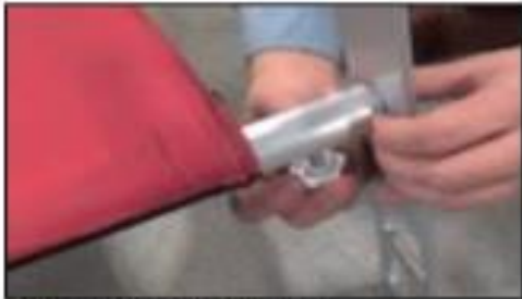
Secure with thumb screw.
