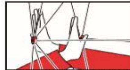
Push on middle hub at back of frame while pushing on corresponding front hub. Instand will sink to the floor. Handle frame at hubs.
