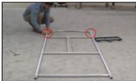
Insert TOP of the frame until button locks engage. *Note: Velcro® strips should face up around the whole frame.
