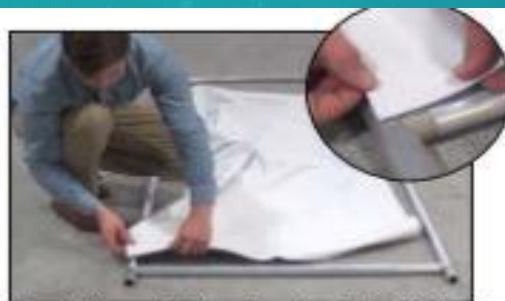
Attach liner to Velcro® at the BOTTOM corner and continue around the frame.
