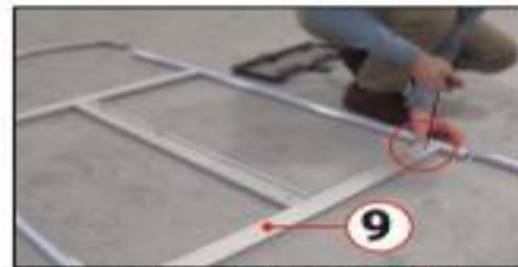
Insert part #9 into hole on the side tube and secure CAM Lock using hex key.
