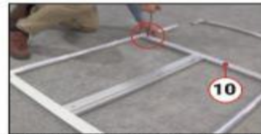
Insert part #10 into hole on the other side tube and secure CAM Lock using hex key.
